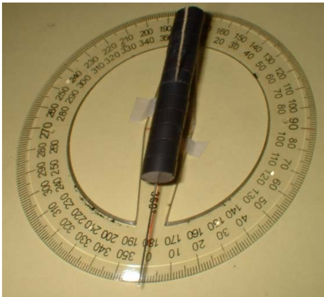
FIGURE 1. Hanging magnet above protractor.
